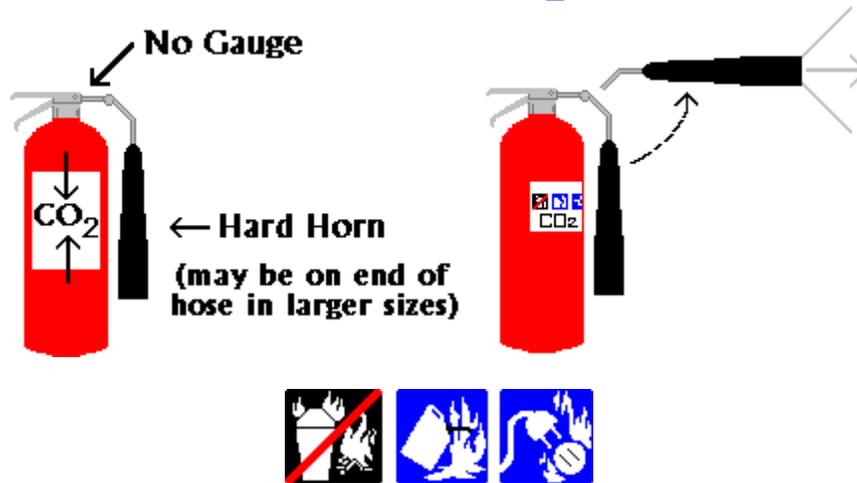
Carbon Dioxide extinguishers are filled with non-flammable carbon dioxide gas under extreme pressure. You can recognize a CO<sub>2</sub> extinguisher by its hard horn and lack of pressure gauge. The pressure in the cylinder is so great that when you use one of these extinguishers, bits of dry ice may shoot out the horn.
